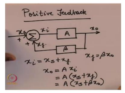
So in the case of positive feedback as I had mentioned a part of x0 is added to the source input Xs ok and proceeding similarly as we had done for the negative feedback case we find that here this xi is = x of S + x of f x of f remains the same and then x of 0 as in the previous case it is = A of x i which is = A of x of S + x of f which in turn is = A of x of S + beta x0 from where we can write the value of x0 in terms of xs as follows.
