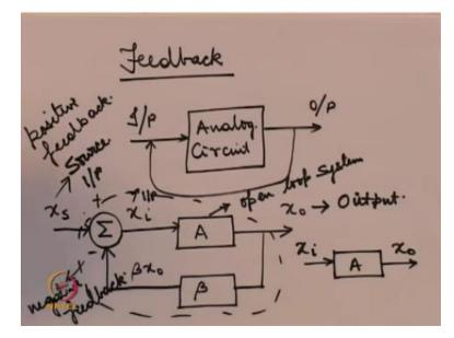
So when I say feedback suppose you have a system, you have an input, you have an output now what feed in feedback we do is we take some of the output and feed it back to the input now it is not that there is some sensing circuit always present for sensing what is the output is just that the circuit is cleverly designed so that this output is automatically fed to the feedback and depending on how we close this loop that is whether it is positive or negative feedback
