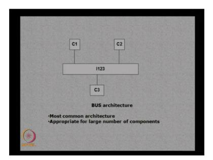
And the other one is the bus architecture which is the most common architecture we can see it in many places this kind of architecture where there be a common interface I123 where I can have one two three is actually here C1 C2 C3 are the components. So, these components can have common interface element. So, I123 represents the common interface between these components.
