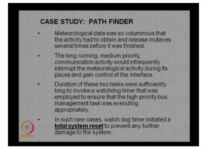
So, this was one of the problem was actually lying in this interface. So, there were many subsystem in the path finder and one of the system was meteorological data or it is actually collection of data from various sensors and passing it to the main system. So,
