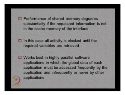
So, the problems with this shared memory architecture is that the performance of this degrades substantially if the requested information is not in the cache memory of the interface. So, whenever that particular information or the variable is not available in the cache memory then it becomes a problem and the performance degrades because it will wait for that data to come or this activity is blocked until the required variables are retrieved.
