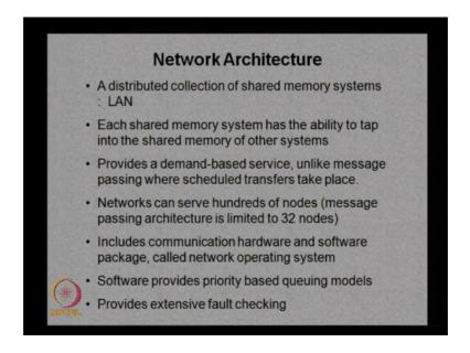
Last one is the network architecture. Network architecture as the name says it is a distributed collection of shared memory system. So, you have multiple shared memory systems in a network that is the network architecture normally the local area network. So, here you will be having multiple shared memory systems. So, we can actually interconnect many shared memory systems to get network architecture.
