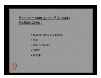
Let us look at some of the network architecture is commonly used in engineering systems. Again as I told you we are looking only at the communication system here as the interface. So, in the network architecture there are most commonly applied or implemented architectures are master slave or pipeline architecture our m bus architecture, another one is the star or spoke architecture, then the ring architecture and mesh architecture. So, these are the commonly used in engineering systems.
