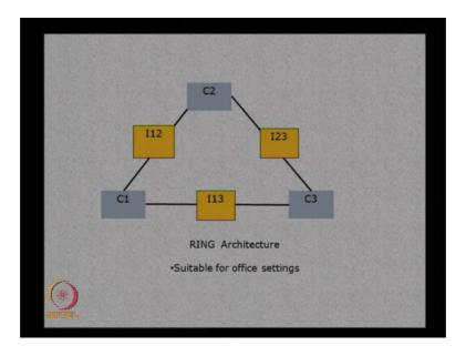
And this is known as the ring architecture which is again it is more like a closed loop control you can have communication between C1 C2 C2 C3 C 1.
