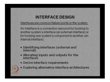
So, this actually shows that interfaces are very important in engineering systems in even a minor error can actually lead to a total reset or the failure of the complete system and therefore, it is necessary for the system designers to look at the interfaces in detail and have a formal procedure to design the interfaces and ensure that interfaces function properly and it actually provides the necessary communication between different some systems.
