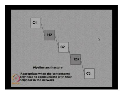
The master slave architecture as you can see here this is a master slave or a pipeline architecture where you have components C1, C2, C3 and there is interface I12, I23 etcetera. So, this kind of architecture allows you to have communication between adjacent blocks or adjacent components. So, C1 can actually communicate to C2, and C2 you can communicate to C3, but there is no other communication possible here.
