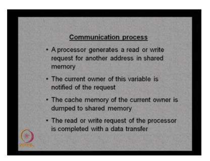
In the communication process in this is basically a processor generates a read or write request for another address in shared memory. So, the shared memory will be having all the address of those nodes which are using the particular shared memory. So, processor generates a read or write request for another address in shared memory whichever system wants to transmit a data to a particular another node. So, it actually generates a read or write request for that particular address.
