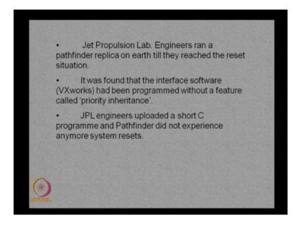
So, the jet propulsion lab engineers ran a pathfinder replica on earth till they reached the reset situation. So, you know to find out what actually is happening in the system the engineers ran a replica on earth till they reach the reset situation then identify the problem that there is a problem with the priorities of each tasks or some task need to be prioritized so that the priority task will always get the mutex and then that will not lead to a error situation.
