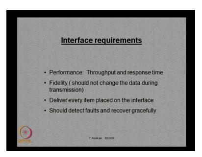
So, the main requirements for an interface is the important performance requirements are basically in terms of performance there are throughput and response time are two important parameters in terms of for interfaces. So, what is the data I can transmit and what is the response time for this transmission, these are the two parameters we need to look at when we design an interface.
