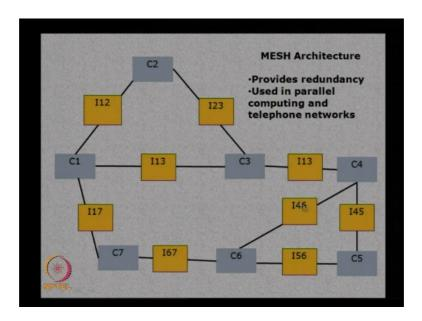
And this is an extension of the ring architecture. So, ring architecture as I mentioned when you have more components then it may not be possible to have ring architecture. So, in this case you can go for mesh architecture.
