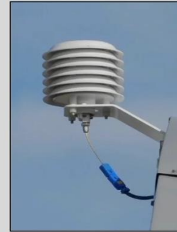
Ambient Temperature Sensor (with radiation shields)
