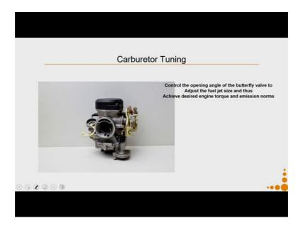
Then comes functional optimization of product components. Say for example, by control so this is a carburettor used in vehicles. So, by controlling the opening angle of the butterfly wall you can adjust the fuel jet size and thus achieve desired engine torque and emission knobs. So, all this can be done using this eco design strategy. So, let us see how to use them and how do I integrate my LCA tool while I am trying to do this activity.
