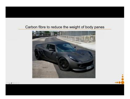
So, talking about reduction in weight. So, say for example, the body of the car it is made up of certain kind of metal alloys. Now, if I take the mechanical properties desired for making these body panels and I find a substitute, so carbon fibre is also plastics reinforced with carbon fibres is a good material for that in terms that it offers higher strength to weight ratio. What it implies is for the strength required the weight of carbon fibre panels is way much lower than the metal panels.
