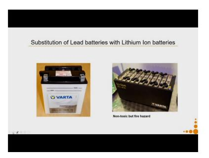
Next example substitution of something which is so when I take a lead acid battery lead acid battery is environmentally hazardous product it has toxicity. So, see if I can replace it with lithium ion batteries. So, the toxicity problem is gone, but there is a fire hazard. So, in case I do kind of a substitution. So, I will have to see how do I build in systems to avoid fire hazard.
