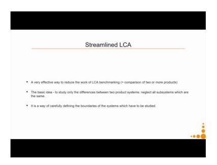
Now, coming to something called a streamlined LCA. What is streamlined LCA? It is an very effective way to reduce the work of LCA benchmarking when you are comparing 2 or more products. So, the basic idea is to study only the differences between the 2 product system neglecting also subsystems which are the same.
