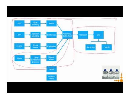
So now again coming back to this particular slide our example of packaging packaged drinking water. So, I can do analysis of say such water that is gate to gate. I can do an analysis of only this phase that is gate to grave. I can do and analysis of the whole system which is cradle to grave. I can do an analysis of only up till the product is produced up till the factory gate which is cradle to gate. Now, let us say can we add more components do it yes of course.
