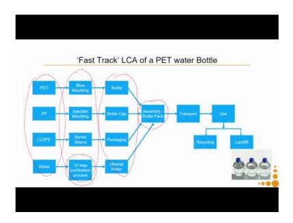
We come back to our previous example of life cycle assessment of the pet bottle. So, in real life scenario most products are in assembly of products or an assembly of components.
