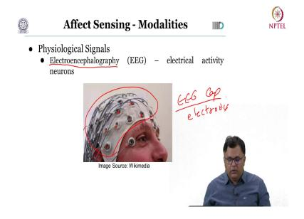
So, that is your Electroencephalography EEG sensor. What is your EEG sensor? Friends you can see here this is a EEG cap ok. What you have here is these electrodes these electrodes and what these electrodes are doing is they are recording the electrical activity in the brain in the neurons.
