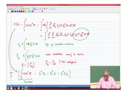
So, the objective function gamma of a particular vector b this is given by integral 0 to T, r of t basically I am expanding the term within this. This will become r of t magnitude squared dt minus integral 0 to T, two times real part of summation K equal to 1 to uppercase K root E k into b K of 1 g K star of t times r of t.
