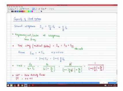
When CDMA and TDMA were sort of completing with each other, the arguments always was which system had more capacity and always argument was CDMA systems have more capacity, and what we are some of the ways in which they were looking at the capacity of a CDMA system. The following is a way capacity of CDMA systems, very very interesting discussion, very very interesting perspective.
