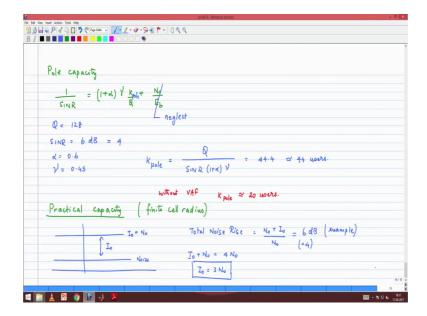
Pole capacity useful for us to write it down in terms of 1 by SINR, I mean easy for us to visualize this. 1 plus alpha times nu K by Q plus N naught by E b, ok. And 1 by SINR; that means usually SINR is a reasonable amount you design your system to have 1 by SINR this nothing but 1 by E b by N naught so this is a small quantity.
