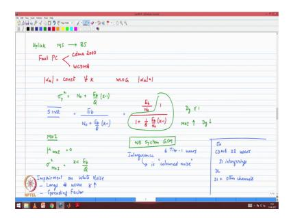
We compared it with narrow band systems such as GSM, where the impairment would be colored noise. Whereas, in this case it starts to with the based on the centre limit theorem, large number of users, the impairment looks Gaussian.
