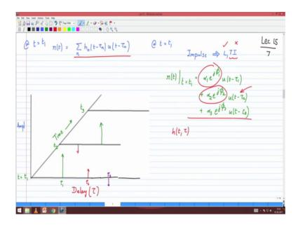
So, a basically I want to write down the expression for r of t, r of t we said was summation over the n the multipath components, h of n t I am going to represent the
