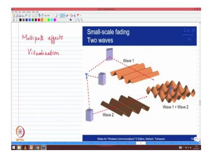
Always very important that we get good intuition, in to what we are working with. So, think of these scenario where the electric field is propagating the signal is propagating in 3, 3 directions from the base station. One is being completely abstracted by one of the buildings. So, nothing propagates behind that another path gets reflected. So, therefore, you get a certain direction of the electromagnetic wave, and then a third direction that is happening.
