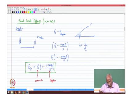
So, that was our understanding of the log normal shadowing. We now move into a after that we went into the effects of small scale. Small scale as suppose the large scale we are talking about changes in the signal which happens when you are moving of the order of 10 to 20 lambda. And one of the things that immediately come into play is that there is a prob Doppler shift of the received signal of the centre frequency of the received signal depending upon the direction of motion.
