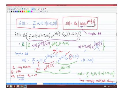
So, a basically the received signal, as we as we mentioned before will be represented in this fashion. This is the bandpass signal. The s of t can have a representation in terms of the baseband signal in terms of u of t. And now what we would like to do is write to the received signal in terms of the modulated signal and then get a base band representation of the signal.
