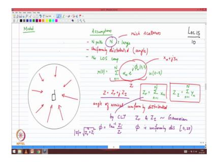
So, now, we move forward to a model that will help us a mathematical model that helps us understanding what is going on this phenomenon. So, basically we will now derive a model, for multipath comp multipath propagation channel where all the multipath components are arriving within the time resolution window.
