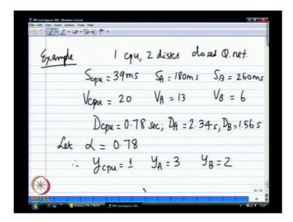
So, now, let us go back to our the same system with queue right 1 cpu, 2 disks closed network. And let us assume that S cpu is 39 milliseconds, S A is 180, S B is 260 seconds, and then V cpu is again given to you.
