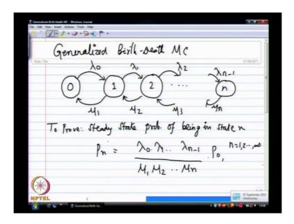
So, this is generalized. So, the characterization is that we have again a set of finite or countable set of states, and the transition rate from state 0 is given by the lambda 0, this is mu 1 and so on. So, the arrival and departure rates are state dependent.
