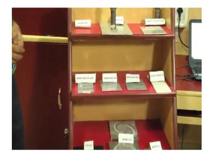
We have got several examples like aluminium and then steel we have got the material you know the one different composites in LAP and (Refer Time: 04:47), you have got the magnesium and then steel, we have also used this HDPE that high density polyethylene, copper and aluminium, and also different configurations including this you know the pipe holding.
