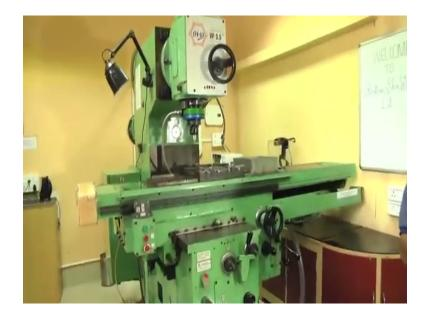
This is the vertical manual milling machine and this machine has got wide range of this spindle speed and this machine has got wide machine or t able as well. And this table can carry the weight up to the 600 kg and the spindle rpm can be up to 31.5 rpm to 6 1800 rpm. And on the same time this table can move along x axis, y axis, z axis (Refer Time: 16:17) 16 (Refer Time: 16:19) per minute (Refer Time: 16:20) to 1600 minute (Refer Time: 16:22).
