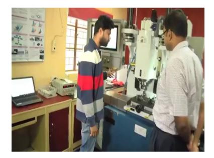
So, behind me what you see over here is a is an indigenous friction stir welding machine which can do friction stir welding on two different materials. So, this particular machine is able to do linear jobs; that means, that two different materials it can weld together in a linear fashion. So, I
