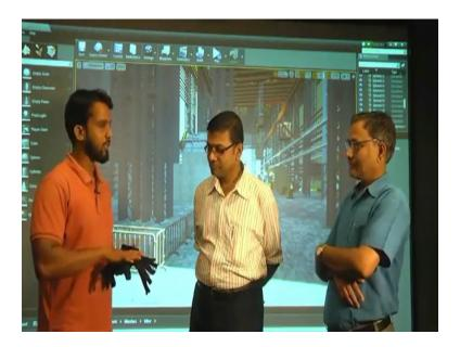
So, we are having different kinds of data gloves. So, these are the data gloves which are used to track all the, used to capture all the motions related to your finger. So, this particular data gloves is having 14 sensors, so it will capture all the finger motions and different wrist motions related to whatever user movement will do; similar.
