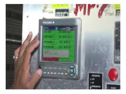
Here we can see the numbers of different type of temperatures of particular milk pasteurisers we can see and from here we can take the data to our to our computers by ethernet connections.
