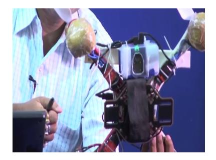
This is a camera this is fitted with a camera, you know over here as you can see this is a camera. And, this UAV could be fitted with cameras to collect images while it is on flight. This particular UAV can and this camera can collect images while it is on flight over agricultural fields to understand different crop conditions and so on and so forth.
