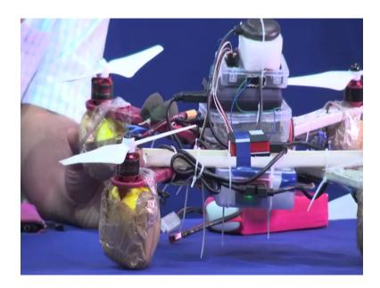
So, as you can see this red colored one is a motor. So, this is this motor right, this is this motor as you can see over here like this all. So, this is this propeller and below it is this motor right. So, like this there are four different motors.
