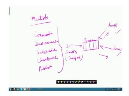
MQTT provides different methods that are used to connect, disconnect, subscribe, unsubscribe, and publish.
