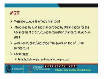
Let us talk about some of the solutions. One of which is the MQTT protocol. MQTT- the full form is Message Queue Telemetry Transport which was introduced by IBM and standardized by OASIS in 2013. MQTT is based on the concept of Publish/Subscribe. This is the key thing over here in MQTT and this works on top of the existing TCP/IP, the way MQTT has been designed to work right.
