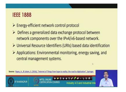
IEEE 1888-this one is an energy-efficient network control protocol, which defines a generalized data exchange protocol between the network components over IPv4 or IPv6. It talks about the use of resource universal resource identifiers and supports different applications for environmental monitoring, energy saving, central management systems, and so on.
