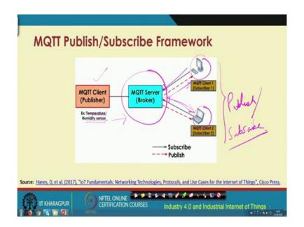
This is an example of how the MQTT publish/subscribe framework works. So, look at this particular picture. We have the MQTT client, which is the publisher on one hand. So, this publisher will publish different sensed data such as temperature, humidity etc. And, this data that will be published in the MQTT broker. MQTT broker, which is a server stores this data.
