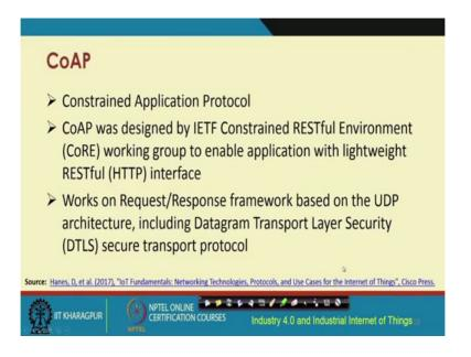
The full form of CoAP is Constrained Application Protocol, which was designed by IETF. The full form of core is Constrained RESTful Environment. So, this particular working group has come up with this core to enable applications with lightweight interface to run in place of HTTP.
