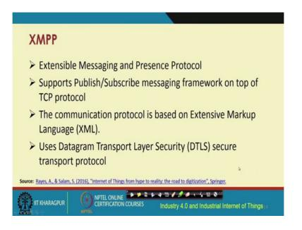
From another point of view, there is another protocol which is called the XMPP protocol. The full form of which is Extensible Messaging and Presence Protocol, which is again based on publish, subscribe, model that we talked about in the context MQTT. The communication protocol, XMPP is based on XML, and it uses DTLS secure transport layer at the bottom in the transport layer for transport layer security.
