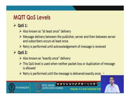
QoS 1: on the other hand, talks about at least once delivery, where retry is performed until the acknowledgement of the message is received. QoS 2 is further different; it is about exactly
