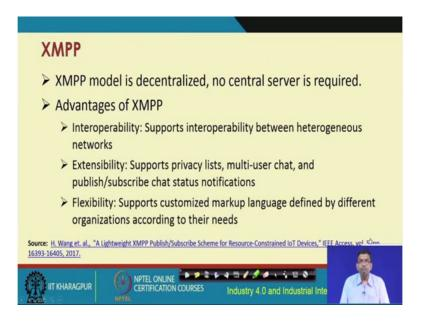
This model is decentralized; that means, there is no requirement for having a centralized server. And, it has manifold advantages such as it supports interoperability between heterogeneous networks, heterogeneous devices, and heterogeneous agents. It supports extensibility; that means, supporting privacy lists, multi-user chat, publish/subscribe chat, status notifications etc.
