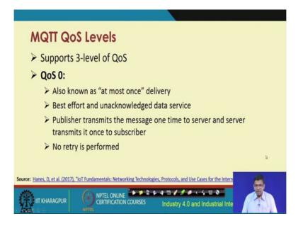
There are different levels of QoS; the first one is the QoS 0 which is about ensuring at most once delivery. So, this is kind of a best effort and unacknowledged data service. And, here the publisher transmits the message one time to the server and the server transmits it one time to the subscriber. There is basically no scope for retry.
