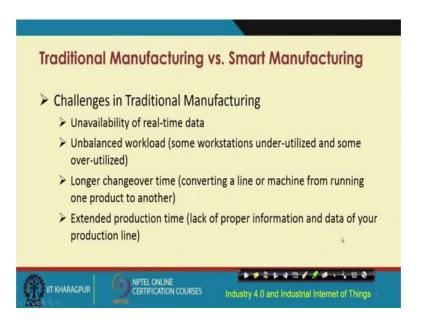
So, whenever we are talking about manufacturing, traditionally there were different challenges, this manufacturing machines deals to work in isolation, these machines were not connected, there were different other challenges such as because these machines were not connected with one another, there was unbalanced work load in this different machines. So, the work load across the different machines doing the same thing was not balanced.
