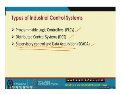
So, there are different industrial control systems that are used for process control. One is the PLC, the Programmable Logic Controller; second is the DCS, the Distributed Control Systems and the third is the SCADA which stands for Supervisory Control and Data Acquisition; Supervisory Control and Data Acquisitions S C A D A. So, this SCADA and SCADA in turn basically use the concept of the PLCs.
