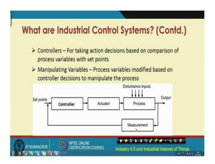
Next comes the concept of the Controller. So, the controller basically takes certain actions. So, based on the process variable based on set point value and so on, it takes certain decisions it or actions and it compares the process variables with the set points before it takes the action. So, this is what this controller does and this is what you see over here in this picture as well.
