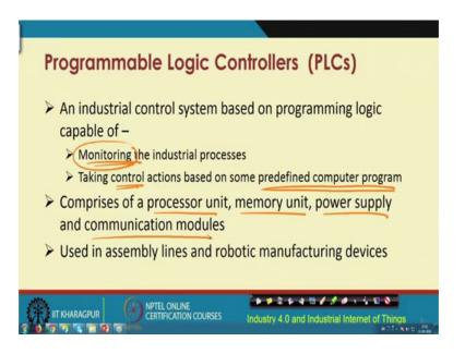
So, what is this PLC? So, basically PLC is the industrial control system. So, it is the industrial controller in control system and this is based on the programming logic of monitoring the industrial processes and taking control actions based on certain predefined computer program. So, the computer program has a predefined set of instructions is provided to the system and based on that the control actions are taken and for that first the monitoring will have to be performed.
