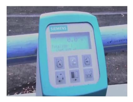
The reading for the flow rate of the through this paddle wheel flow meter will be displayed here and also the total amount of water passing through this flow meter over a period of time will also be displayed here.
