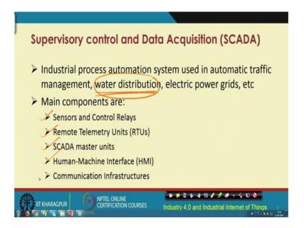
So, this kind of device SCADA based device basically is helpful in order to achieve the requirements of industry 4.0. So, industrial process automation systems are used in automatic traffic management, water distribution then, electrical power grids and so on and in this particular lecture, I am going to show you the case study of use of SCADA in water distribution system, but it could be used in other plants also.
