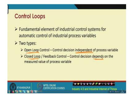
So, we let us look at this Control loop because it is this control loop which is the attractive part in the whole process control automation and so on. So, this control loop is the fundamental element of industrial control systems and this basically these control loops help in automatic control, unmanned autonomous control, automatic control of industrial process variables is offered with the help of this control loop.
