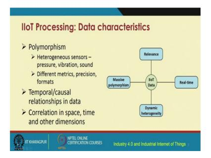
How we can deal with this data, we need to first understand the type of data, that we are receiving. The type of data, that we receive can be characterized in different ways. First of all this data has massive polymorphism in place. Massive polymorphism means, we are talking about the use of large number of different types of sensors, pressure sensors, vibration sensors, sound sensors, and large number of different types of sensors could be used.
