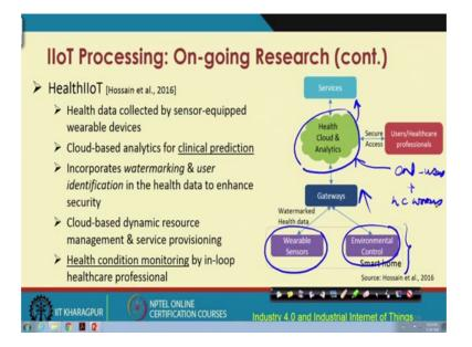
Hossain et al. came up with the health IIoT solution. And this is this solution they came up with, in their architecture they are talking about smart homes. They consider the smart homes, they consider the use of different wearable sensors, which could be owned by different humans, and also the use of different environment control sensors at homes.
