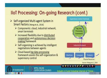
So, in another work by Wang et al. they came up with a multi agent system for smart factories, where they are talking about use of physical resources at the very bottom layer. These physical resources like machines conveyors and the products they are going to be sensor-equipped and are connected to one another. So, through the industrial network the data are going to be coming for centralized event, centralized processing.
