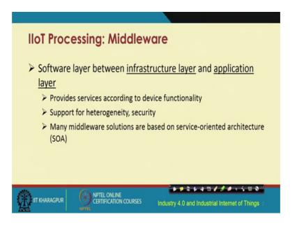
So, it is proposed that we could use some sort of a middleware. Middleware means it is a software layer, which will be standing between the infrastructure layer and the application layer. So, this particular middleware software will provide different services according to the device functionalities. This middleware could also implement security
