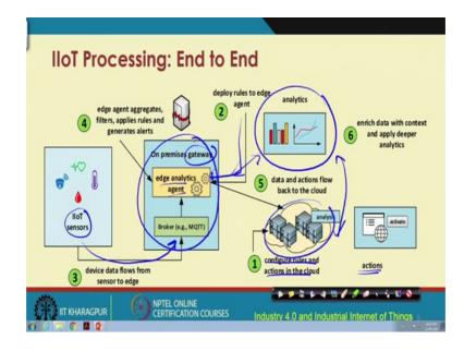
So, let us look at this end to end mechanism and let us try to highlight stepwise, how this processing is coming into picture and its importance. So, let us look at this particular figure and as shown over here. We are talking about; we are talking about different steps; step one is configuring the rules and actions in the cloud.
