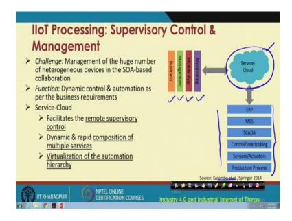
So, there are different solutions, that are placed that are in place, with respect to analytics and processing. So, one of the solutions the source is given over here. So, this particular solution was proposed by Colombo et al, talks about supervisory control and management in the context of processing. So, as we can see over here its 3 different components in this particular solution mechanism.
