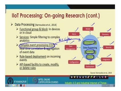
Karnouskos came up with another solution for data processing. So, for data processing they have different components, they have the service engine, a calculation engine, and filtering component. So, all of these things are going to be done at the data processing engine. Service computation, calculation of different types of computation etcetera and filtering all of these are different components of this data processing engine.
