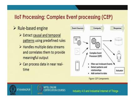
So, let us look at this complex event processing. So, one of the ways to do it is with the help of a rule based engine and this is shown over here in this particular figure. So, let us look at the complex event processing, one of the ways to implement it is using rule-based engine.
