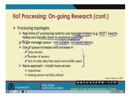
Another work by Dey et al. they talk about the use of different processing topologies. So, here they are talking about real time IOT processing systems using some kind of message broker. Message brokers such as MQTT, which we have studied before or similarly Apache Kafka could be used as message brokers in their system. And those could be used to transfer the data to different analytical pipelines.
