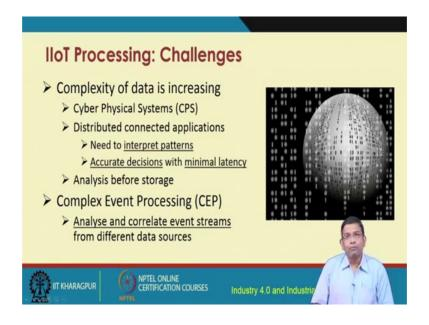
Now, the so, we have to process the data, but there are different challenges with respect to this processing. The complexity of data in industrial systems is increasing day by day. These industrial systems exhibit the behavior of cyber physical systems, where there is an intricate relationship, that is there between the cyber component and the physical component of the different machines and there and the interconnected ones.
