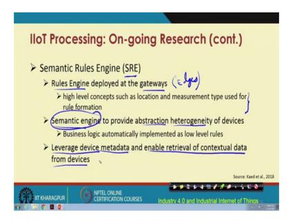
Kaed et al. talked about the use of semantic rule engines SREs, Semantic Rule Engines. These rule engines are deployed at these different gateways or the edges. So, these rule engines are going to do some kind of high level processing, with respect to the location and the measurement type, that is used for rule formation. So, this preliminary level processing is going to be done by the rule engine.
