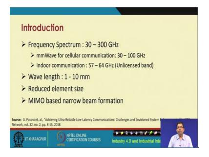
Then comes the millimetre wave communication, where the communication happens in this particular band of the spectrum 30 to 300 Giga hertz band and this basically
