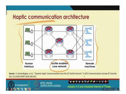
Haptic communication architecture is given over here. So, we have this human interface we have this human interface, this is this human interface we have these remote machines and in between we have this tactile enabled core network and this overall haptic communication architecture is shown over here.
