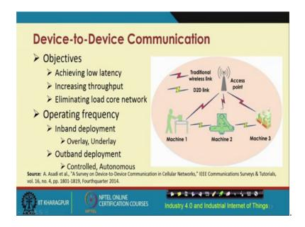
Device to device communication here we are talking about this kind of thing. So, machine 1, machine 2 they can talk to each other D2D link, again machine-to-machine 3 another D2D link device-to-device communication that basically cuts down on the time or the latency of communication and so on. So, these are the D2D links this is one, this is another and we are talking about it in contrast to the traditional links.
