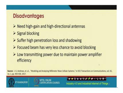
So, disadvantages of millimetre wave communication is that there is a need for high gain, and high directional antennas, and there are different other disadvantages such as have this technology suffers from high penetration loss, and shadowing, and there are many different disadvantages.
