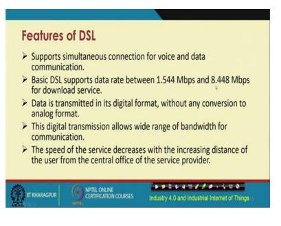
So, the basic DSL supports data rate of 1.544 Mbps and 8.448 Mbps for download surface. Data is transmitted in digital format, without any conversion to the analog format. And, this digital transmission allows wide range of bandwidth for communication.
