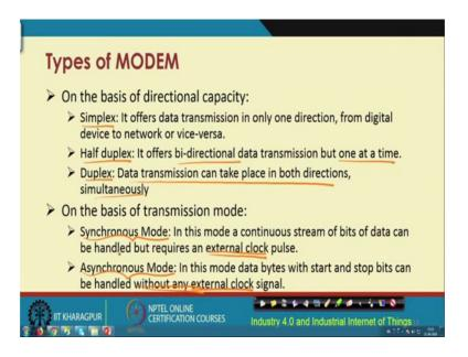
So, there are different types of MODEMs that are supported; simplex modem, half duplex, and duplex. Simplex offers data transmission in one direction, half-duplex
