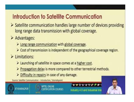
Satellite Communication is a well-known technology, for offering global, long range, communication between different points, but these satellite communication devices come at higher cost. There is higher cost although, it is much more effective in providing global coverage in terms of communication, but the cost of these devices is much higher.
