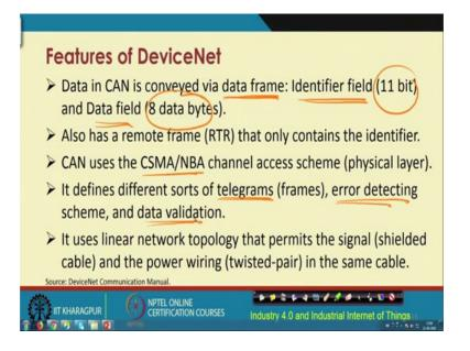
So, there are different features of DeviceNet. The data in Controller Area Network is conveyed with the help of data frame. So, this is nothing new so, in the form of frames. These frames have this id field which is of 11 bits and the data field which is of 8 bytes.
