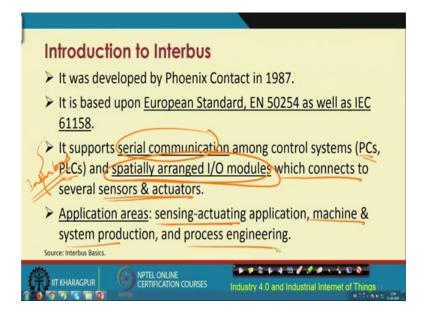
Next, comes the inter bus protocol. So, this particular protocol was developed in 1987 by the company phoenix contact. It is based on the European Standard, EN 50254 as well as the IEC 61158. Supports serial communication, in this case, serial communication between PCs, PLCs and specially arranged I/O modules, and these specially arranged I/O modules will in turn connect to different sensors and actuators.
