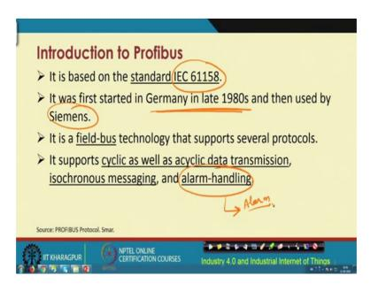
The next one is the Profibus protocol, which is basically the process field bus; this is the full form the process field bus Profibus protocol we are going to go through now.
