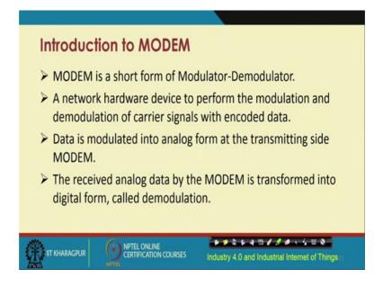
MODEMs are quite popular, MODEM technology, MODEM stands for Modulator-Demodulator, which is basically a device that will do modulation and demodulation of carrier signals, with the encoded data. And, this data is modulated into analog form at it is transmitting site and the received analog data, by the MODEM is transformed into the digital form at the demodulator side.
