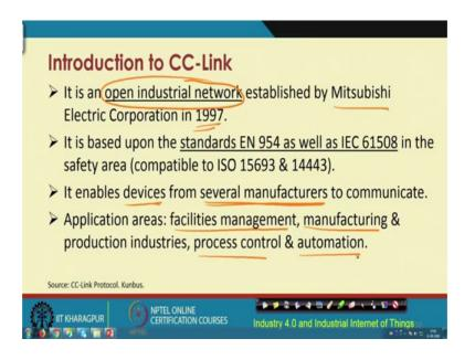
Next comes, this protocol the CC link CC stands for Control and Communication. Control and communication link protocol, CC link. This is basically an open industrial network protocol. So, here actually we are talking about all different types of protocols, different companies came up with Siemens, Mitsubishi electric corporation etcetera.
