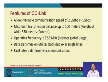
So, overall the communication speed is quite varied in CC link 2.5 Mbps to 1Gbps, transmission distance that is supported is 100 meters for field bus and for control 550 meters, operating frequency is 13.56 megahertz. And, it supports both duplex and data transmission in the form of duplex, and single transmission lines. And, overall the deterministic communication is supported by CC link.
