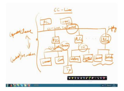
We have the controller devices, the master devices, these slave devices will be operated by different operators and these master devices by the controllers.
