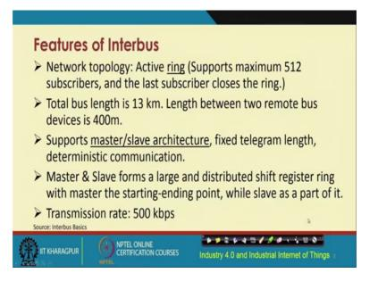
In terms of other features, network topology that is supported is the ring topology, which will provide connectivity to about 512 subscribers. The total bus length is 13 kilometres, which is quite long as you can see. So, 13 kilometres of operation is quite helpful for industrial requirements. Master slave communication architecture like, before is still being used and the transmission rate that is supported by inter bus is 500 kbps.
