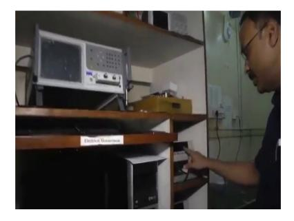
So, we have two electrometer here, one is a source measure unit and another one is a very high resistive measurement type electrometer. So, usually we use this electrometer to measure the transient that is the base data that we measure so these are all dc measurements. So, we have the capability to go for AC measurements. So, we can do the impedance spectroscopy, by this impedance analyzer and that will tell us that; what is the difference between; a DC measurement and AC measurement.
