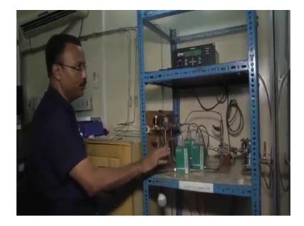
And so the gases that are coming from the many fold there are four different lines. And one exclusively we use for the carrier gas and in most of the instances the carrier gas is here, which is having 20 percent of oxygen and a variety of test gas. So, this gas controlled this gas they are controlled by this mass flow controller. And at present there are three mass flow controller and we can add 1 or 2 more and this is controlled by this controller.
