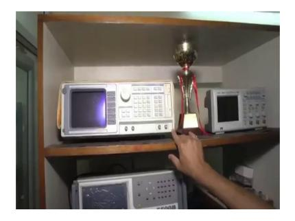
And also we have another network analyser, which basically we use for noise spectroscopy, because sometimes are noise inside the resistance transient that also gives lot of information. This is not very frequently used, but this gives very very exceptionally high quality data as per as understanding of the types of gases concerned. Because basically when you measure the resistance versus time the data is more or less very monotonous.
