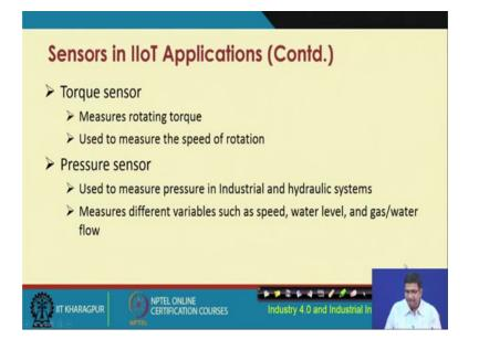
Other industrial sensors are like torque sensor, pressure sensor, vacuum sensor, acceleration sensor, speed sensor, PIR sensor.
