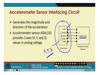
Then we will have a look at another very commonly used industrial sensor, which is the accelerometer sensor, and this is this accelerometer sensor that is shown over here the this is basically how this ADXL335 accelerometer sensor looks like and these are the different pin configurations. These accelerometer sensors are connected to a microcontroller in this manner, the first one corresponds to this VCC the maximum voltage of operation.
