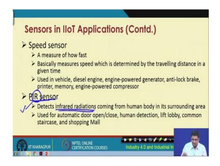
PIR sensor basically detect the infrared radiation coming from the human body in its surrounding area it is used for automatic doorbell, close closer, human detection, then the elevators in the lobbies, then common staircase, and shopping malls. PIR sensors are very commonly used, IR actually stands for infrared. So, these are basically based on infrared radiation.
