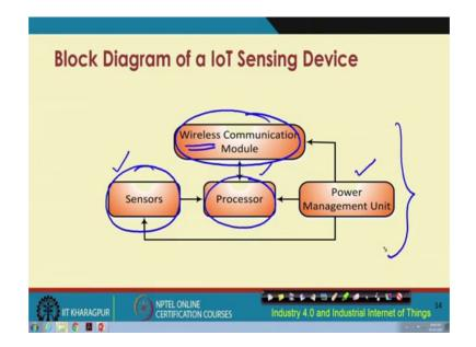
So, going back we have seen that these sensing devices are very important. So, these sensing devices have the sensor, which will which is actually the element, which is
