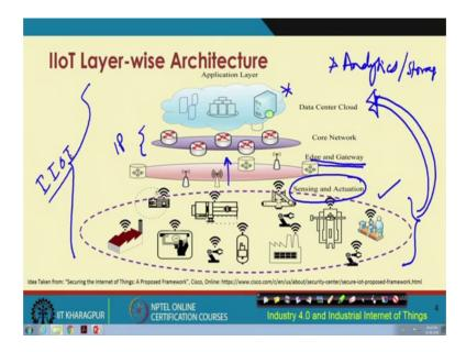
So, we need to understand this part in more detail so, if we look at the IIoT, if we look at holistically. This smart sensing element, the smart sensors are basically at the very bottom. So, we have these different smart sensors and actuators in the bottom most layer.
