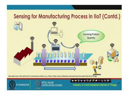
Then the product moves on comes to this particular point, where the counting of the number of units of production, the units, which have been not only produced, but tested over here this counting takes place counting of these products takes place. And then this data again is sensed is sensed and is sent over here to that intermediate node, this intermediate node again sends it to the central processor for further processing and storage this information.
