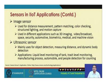
The we could also have other types of sensors like image sensors, ultrasonic sensors like based on sending ultrasound, sound waves are sent these are ultrasonic sensors are also commonly used for object detection, measuring distance, dynamic body detection, liquid level monitoring of tanks, trash monitoring, manufacturing process, automobile, people detection.
