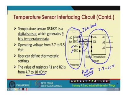
As I was telling you that temperature sensors are very important I have shown you an analog temperature sensor, but we could also have digital temperature sensors. The functioning of a digital temperature sensor is bit different from the way, the analog sensors work. This is an example of a digital temperature sensor, the model is DS1621 and this particular sensor will generate 9 bits of temperature data and this sensor digital sensor operates in the range 2.7 to 5.5 volts.
