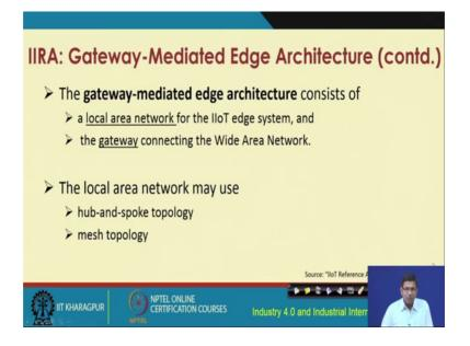
So, like the previous architecture here again let us go through each of these architectural components of the gate gateway-mediated edge architecture, in further detail. So, this gateway mediated edge architecture consists of a local area network for the IIoT edge system and the gateway connecting to the wide area network. The local area network may use a hub and spoke topology or, a mesh topology.
