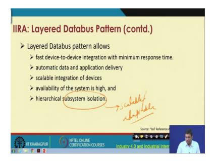
Layered databus pattern basically allows first device to device integration with minimum response time, automatic data and application delivery, scalable integration of devices, availability of the system making, it higher and hierarchical subsystem isolation. So, this isolation part is very important subsystem isolation, because this will help in making the solutions much more scalable and adaptable, adaptable to what; adaptable to different changes.
