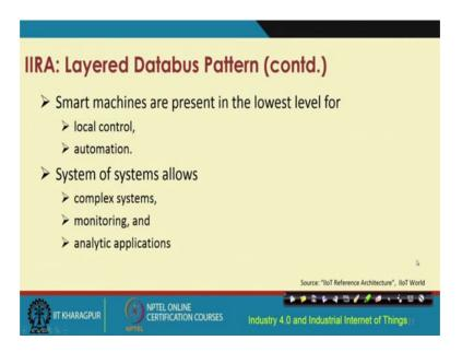
Let us go through this pattern also little bit, in further detail. So, here we are talking about use of smart machines. So, these smart machines at the lowest layer will help in local control and automation processes. System of systems layer allows complex systems to be executed, complex monitoring, complex processing, and analytic applications, all of these things could be executed at this particular layer.
