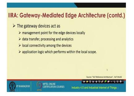
So, you have this local area network, which supports two different types of topologies, the mesh topology and the hub-and-spoke network topology. Then you, we have these gateway devices acting as the management points for the edge devices locally transferring helping in the transferring of the data, processing of the data, and analysis of the data.
