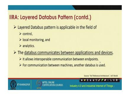
Then you have the layered data bus pattern, which is applicable in the field of control local monitoring and analytics, and the database basically communicates between the applications and devices through this communication is enabled with the help of the data bus. This communication will essentially help in allowing interoperable communication between different endpoints, between different machines.
