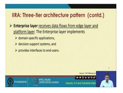
And finally, the enterprise layer concerns receiving data flows from the edge layer and the platform layer. So, I mean directly from the edge layer, the enterprise layer could be receiving the data or it could be from the platform layer, which again receives the data from the edge layer. So, the enterprise layer basically implements domain-specific requirements, decision support systems, and other requirements such as interfaces to end-users.
