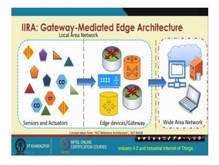
The next type of architecture is the gateway-mediated edge architecture. Here basically we are talking about incorporation of the, the gateway, gateway concept. So, we have all these different sensors and actuators, these sensors and actuators throw in lot of data. And through the different gateway devices, edge devices, gateway devices and so on the data are sent to the wide area network for further dissemination of different information and so on.
