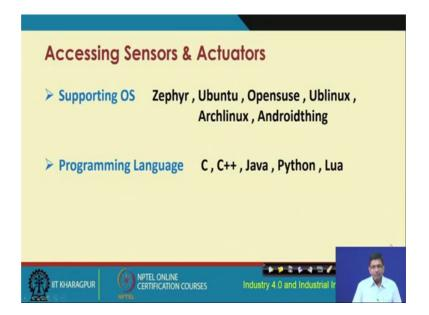
So, there are different sensors which would sensors and actuators industry scale which would support different operating systems, such as the ones that are mentioned over here. Zephyr, Ubuntu, Opensuse Ublinux, Archlinux, Androidthing, these are some of the different operating systems that are used in the smart sensors and actuators.
