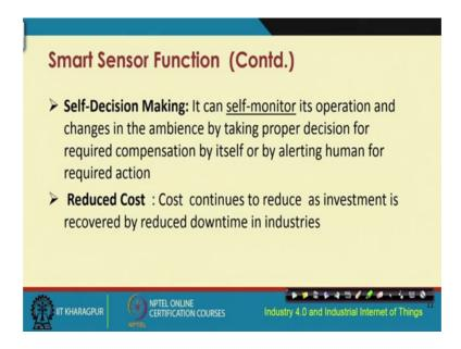
So, the next important function is the self-decision making. Because it is a smart sensor, an intelligent sensor, it has to do things on it is own. So, it has to self-decide, it can self-monitor, and based on the ambient conditions, it can make certain decisions on its own. And this would be possible with the help of the processor that is inbuilt into this smart sensor.
