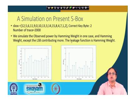
So, here is a further example on a present S box. So, present s box is being denoted here. So, in this case the correct key byte is at specific location the number of trace is 2000. Again you see the now right you can get a corresponding peak. So, in this case the leakage is modelled again by the hamming weight and we indeed get a corresponding peak at the corresponding key guess value.
