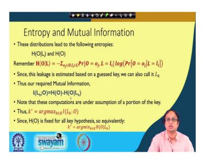
So, the corresponding entropy is there for now given by this formalism. So, therefore, suppose I want to calculate. So, we are all said to calculate H O of L i O given L i and also H of O. And therefore, we know that H of O given L is nothing, but this probability estimation. So, there it is probability of O equal to O j comma L equal to L i multiplied with log of probability of O equal to O j given L equal to L i.
