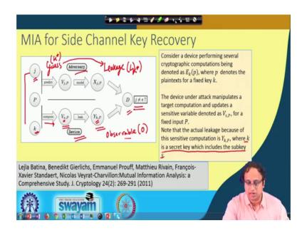
So, now, with this background let us see and try to see how we can apply MIA for side channel key recovery. So, here is one very fundamental paper from published in journal of cryptology in 2011. So, this diagram is taken from this paper. So, you can observe that what we try to do here is there are certain random variables which are being defined here.
