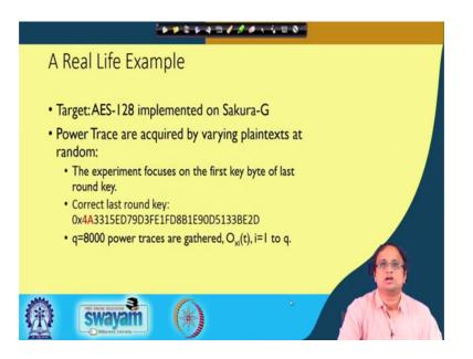
So, here is a real life example where we basically target an AES-128 implemented on a Sakura-G platform and the power trace which is acquired by varying plaintext at random the experiment focuses again. So, this is my correct key this is a 128 bit key and I again focus only on the first key byte. So, we take 8000 power traces ok.
