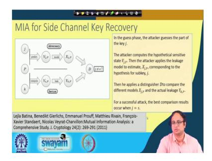
So, therefore, here is the remaining part of the attack. So, in the guess phase so, therefore, the previous one was the you know like when you are profiling and you are getting the observable O and now you are trying to estimate the leakage s I mean the leakage L. So, this is a guess phase and in the guess phase the attacker guesses the part of the key say j and the attacker computes the hypothetical sensitive state V j, P.
