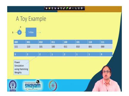
So, now let us try to apply this on a toy example. So, this is a toy example of an S box which is nothing, but you know like this is a mapping which is it is just a symbolic box. So, what we do is that we basically model the power based on the hamming weights. So, you can see here the hamming weight 3 means it is written the observable is 3. This is the hamming weight is 2 so, the observable is two the hamming weight is 2 the observable is two and so on.
