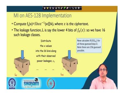
We observe the corresponding observables O and then do a similar mutual information of analysis attack. So, therefore, what we do is we calculate we are doing from the cipher text now. So, therefore, we do S box inverse of x XOR k where x is a cipher text. Now
