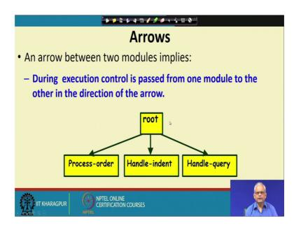
The second element of a structure chart is the arrows the arrow represents the invocation relation that is which module call switch module. And when there is a call from one module to another module, then the control is passed from one module to the other. So if root calls process order then the control is passed from root to the process order and then once the process order completes the control is back with root and then it may call handle indent and then the handle query.
