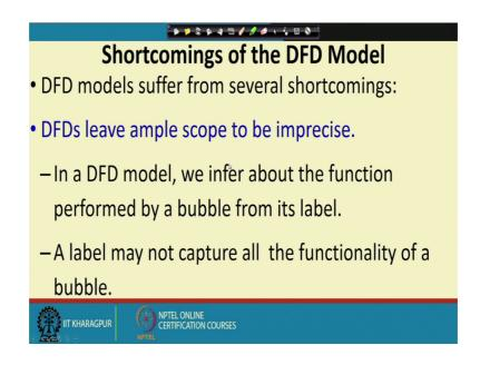
The first difficulty is that here the functions are only identified by the names written on the bubble. And therefore, can be very imprecise, just by looking at the label we have to in firm infer about what all is involved in the function and therefore, many things will remain ambiguous incomplete.
