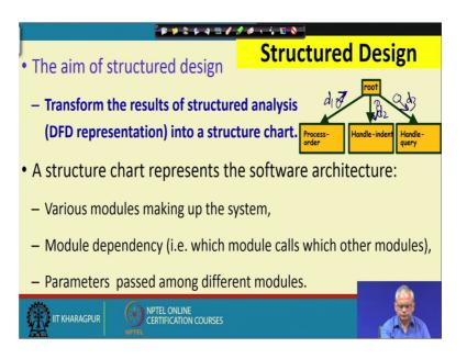
So, this is an example of a structure chart of a problem and we will have these are the modules of our design and for each we will write a module in the code. It represents the call relationship between 2 modules, so the root calls all these 3. We will also represent the data flow that occurs between the different modules through a some notation we will see, we will write the name of that at a d 1, d 2 and so on.
