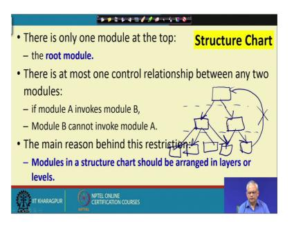
Now, the structure chart there will be only one module as the root and then there are control relationship between two modules. If the module invokes the other module and based on the methodology that we give and also any structure design methodology we always come up with a structure like this. It is a tree like structure these are arranged in levels, but then we do not have lower level module calling a higher level module we do not have this kind of arrow here.
