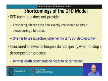
We already seen that how to decompose, that is not clear we just say that see bubble should be decomposed in the next level. Take 1 bubble from a layer level and then decompose it.
