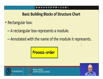
Now, let us see what are the basic building blocks of the structure chart of course, the central part of a structure chart at the modules. The modules are rectangles and the name of the module is written very simple that we draw a rectangle for each module and we just write the name of the module on the rectangle.
