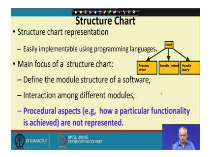
Now, let us see what are the elements of the structure chart, the structure chart identifies the module structure and we can easily program the structure chart. It is actually the high
