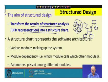
Now, once the data flow diagram model is complete, based on the model we develop the design the high level design and we call the process as the structure design. The structure design it takes the results of the structured analysis and it transforms this structured analysis into a structure chart. So if this is our set of DFD's the DFD model as you are saying is consists of a set of data flow diagrams the root level, level 1, level 2 diagrams and so on.
