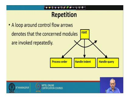
One more element here is the repetition on the invocation arrow if we draw an arc shaped arrow here that indicates that these modules are called many times; in a loop.
