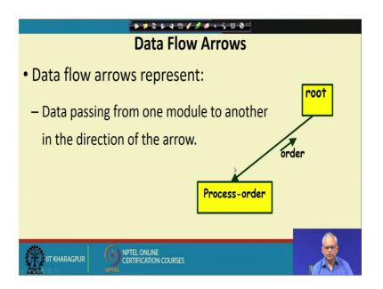
The third item or the third element is the data flow. So represented here the data flow aspect we draw a arrow here on this invocation showing the direction of the data flow. So what this represents is that the root calls the process order and the process order gives back the order to the root, very simple notations.
