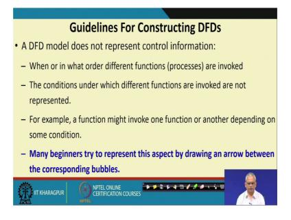
This is one of the very common problem. They represent the control arrows here, that is which one operates after which one and so on and that is not correct..
