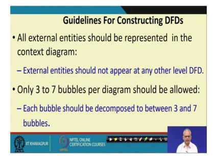
The external entities appear only in the context diagram and in level 1, level 2 etcetera context, the external entity should not appear. In any DFD level only 3 to 7 bubbles per diagram should be allowed.
