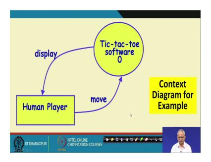
So, that is the context diagram very simple here, that write the name of the software Tictac-toe software, number is 0. The external entity is human player, enters, moves and receives the display. Now, how do we develop the level 1 diagram? In the level 1 diagram, we identify the high-level functionalities and represent them as bubbles typically between 3 to 5 bubbles in the level 1 diagram.
