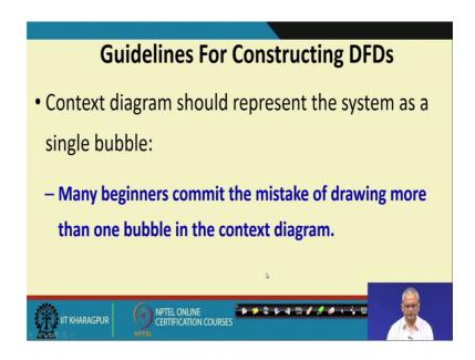
Now, let us see some of the mistakes to avoid while constructing a DFD. The context diagram contains only one bubble, that is the simplest representation. If we draw more than one bubble in the context diagram that is not correct.
