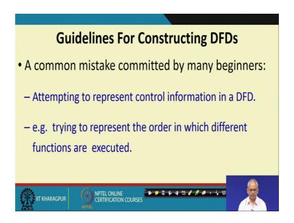
Here only the data flow is represented, we should not represent things like which one which function operates before which other function etcetera. We just represent here each function, what data it needs and what data it produces.
