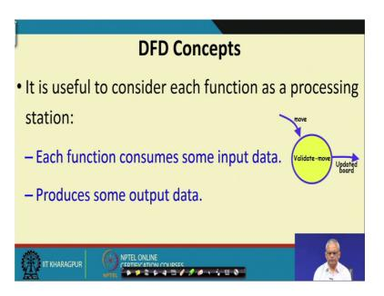
As we were just saying that each a function is represented using a circle and this represents some processing. It takes some input data, does some processing and produces some output data.
