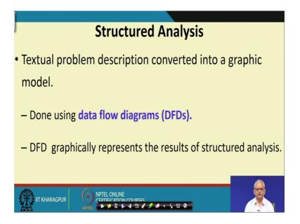
For doing the structured analysis we will use the DFD technique. DFD stands for data flow diagrams and this is a very intuitive and simple technique. It takes hardly few minutes to get familiar and get productive and get started using this technique.
