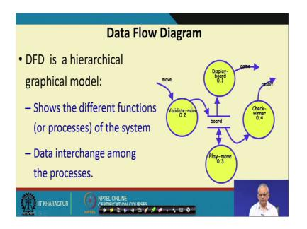
And it is a graphical technique, we will use the DFD which is also called as bubble chart to represent our result. The DFD allows us to do a hierarchical decomposition and that is why the DFD is a hierarchical graphical model, we will have various levels of model. Some are very high-level model and then these are further decomposed into finer or more detailed levels.
