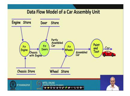
The model is extremely simple as you are saying without much effort we can easily understand a model developed using this, just let us look at this car assembly unit modeled using the DFD notation. So, here the processes fit engine, fit door, fit wheel paint and test; you can observe here that each of the process represents some activity and that is why these are starting with the verb form fit engine, fit door, fit wheel, paint and test.
