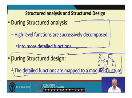
So, now let us get into our discussion on structured analysis and design. So, here as we are saying that we will start with the high-level functions as specified in the SRS document and then we will decompose into detailed functions. So, that we will call as the structured analysis. So, this is the structured analysis activity where we do a functional decomposition.
