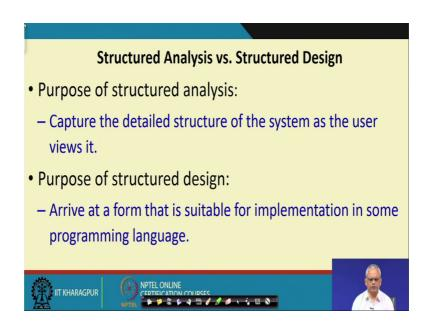
One thing we must be clear is that the structured analysis is just a elaboration of the things that the customer wants. On the other hand in structured design we arrive at a form that can be easily implemented that is coded into a solution. Obviously, the form structured analysis if you are done the structured analysis we cannot derive a code from
