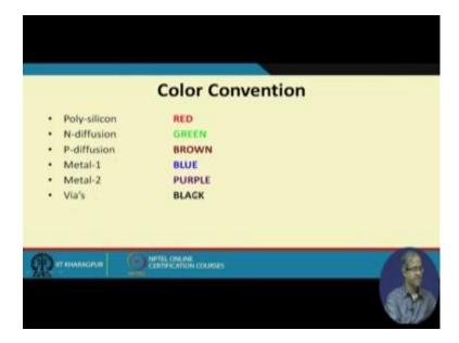
These are the conventions that I had talked about. So, a polysilicon wire is represented in red diffusion for N type diffusion is green P type diffusion in brown, metal 1 blue, metal 2 purple and the Via's the connections contact represent black.
