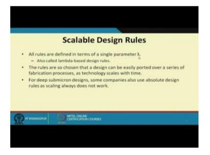
Now most of the design rules that have been used means in practice they are sometimes called scalable. Scalable means this rules are defined in terms of a parameter lambda.
