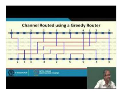
And of course, we will need additional tracks if required, and if you follow this heuristics this is just an example which has been worked out I suggest that you work it to out by hand, and see how it works we do it like this from left we go on starting from one assign to the same track.
