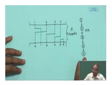
Suppose we have a vertical constraint between 1 and 2, say between 2 and 3, 3 and 4 and say 4 and 5. So, here though there is no cycle, but there is a long chain in the vertical constraint graph 1 to 2, 2 to 3 and 3 to 4.
