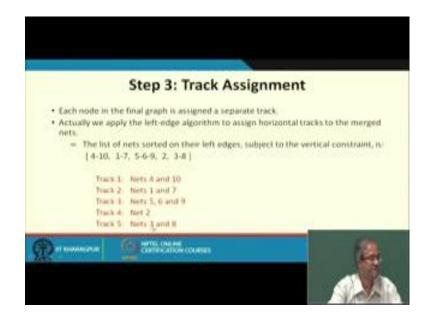
So, last step track assignment you do it according to that. These are the vertices in the graph first track you see now you just order by the vertical constraint graph, you have to take 4 10 first no incoming edges, then 1 7, then 5 6 9 these 2 can be done in any order 2 and 3 point at any order.
