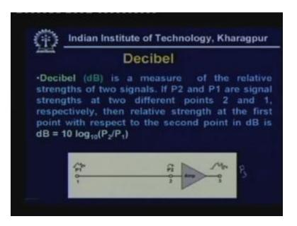
As shown in this diagram for example this is the point P1 from where the signal is passing and it is going to point P2 and as you can see this was the signal sent and at point P2 it is very much attenuated. Now we use an amplifier between point 2 and point 3 and we get an amplified version of the signal.
