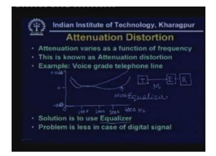
Here the voice grade telephone line has bandwidth from 0 to maybe 4000 Hz. This is your 2000 Hz, this is your 1000 and this is your 3000. And on this side we draw the attenuation and this is 0 say this is minus 10 dB in decibel and this is plus 10 dB. The bandwidth of the medium that means the voice grade telephone line in this case can be represented like this. Here it is shown as 100 KHz that means with respect to hundred KHz it is 0 so it will be somewhat like this.
