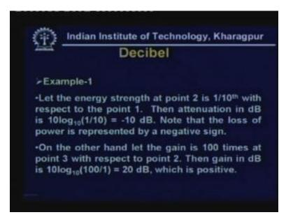
Now let me explain this with the help of an example. Let the energy strength or power at point 2 is 1 by 10 with respect to point 1. Then attenuation in dB is  $10\log_{10} 1$  by 10 that is minus 10 dB. It may be noted that the loss of power is represented by a negative sign. So we find that whenever there is attenuation by looking at the sign of that decibel value we can find out the level of attenuation and also you can identify that it is attenuation.
