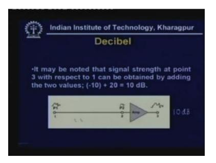
So here with respect to point one the amplification is 10 dB. So we find that finally from here to here if we consider then it is not attenuation but a gain of 10 dB. So in this way the decibel values can be added whenever we have a number of devices or channel in cascade to find out the final value of attenuation or amplification whatever it maybe.
