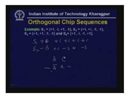
Whenever you have got some stations not sending even then it will work. That means in this case if some station is not sending data, consider this is not here (Refer Slide Time: 40:37) that means B is not sending, this is dash so in that case it will be  $0\ 0\ 0\ 0$  even then it will work. That means if it is  $0\ 0\ 0\ 0$  and if you do the summation you will find still at the receiving end you will be able to detect by proper addition.
