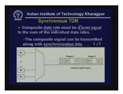
Here are the buffers coming from different sources and here you have got some kind of switch so a connection is established between S1 then S2 then in this way up to Sn but it is done very fast and some kind of framing is done and composite signal is framed where you have got data from S1 S2 up to Sn likewise it is repeated so again another frame comes up as S1 S2 and Sn.
