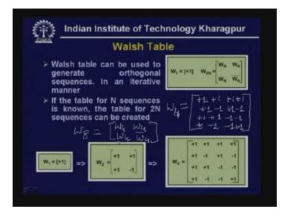
So in this way you can generate the next bit sequences in an interactive manner. So, if the table for n sequences is known the table for 2N sequences can be created and it can be proved that these sequences satisfy the orthogonal property. So this can be used for the purpose of CDMA and also the codes can be generated very easily and these sequences can be also generated by using linear feedback shift register as I have already told.
