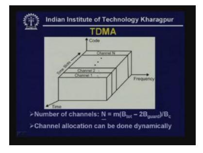
So, as you can see here the frequency and code remains same for each of the channels however the time slots are varying. In this case the number of channels is equal to N where m is number of bits for each of the stations multiplied by B total that is the total bandwidth available minus two into the guard bandwidth by  $B_c$  the bandwidth of each of the channels so you have got separate channels.
