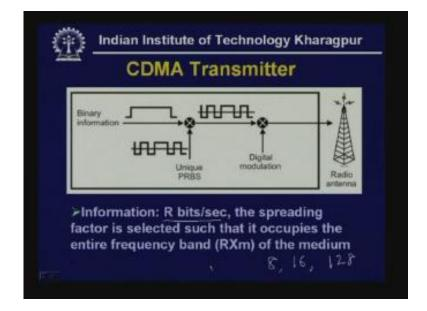
That means the number of bits in this chip sequence is chosen such that it occupies the entire bandwidth of the channel. So it can be 8, it can be 16 or it can be 128 depending on the bandwidth of the medium. Therefore, the signal that comes out becomes m times which is the number of bits in the chip sequence the data rate of the medium.
