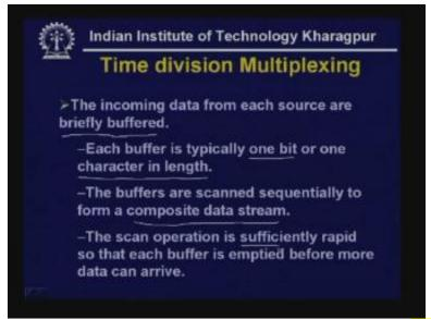
As you know the incoming data from each source are briefly buffered. We have already discussed the Time Division Multiplexing at length and we have seen that each buffer is typically either one bit or a character in length. The buffers are scanned sequentially to form a composite data stream and the scan operation is sufficiently rapid so scanning is done very fast so that each buffer is emptied before more data can arrive. Here it is shown how it is being done.
