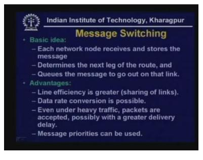
That means here for example this may be a slow link (Refer Slide Time: 8:38) A to this particular node 1. So here data rate transfer can be small on the other hand whenever it is sent from node one to node two data can go at much higher rate. Not only can it go at much higher rate if one can use different encoding techniques.
