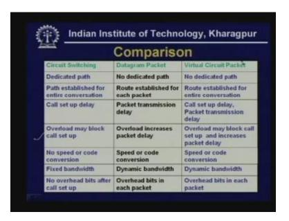
Now we have come to the conclusion part of the lecture where we are comparing the three techniques; circuit switching, datagram packet switching and virtual circuit packet switching because these three techniques have been merged as the key techniques used in switched communication network. Hence in circuit switching we have seen that a dedicated path is created from source to destination and that path remains valid and is used for sending the message.
