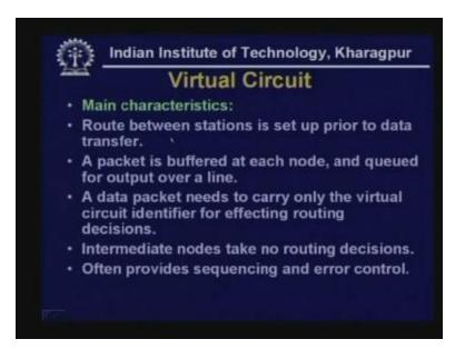
Another point is it often provides sequencing and error control. Some kind of sequencing and error control may be provided in that case CRC is provided and suitable ARQ technique can be used.
