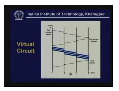
Again they call request packet goes to the next node (Refer Slide Time: 18:15) and ultimately the other side will send call accept packet and call accept packets are also stored and forwarded just like any other packet it goes in the reverse direction and when it reaches the source node where the packets are originating the packets may be sent one after the other.
