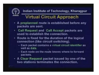
In virtual circuit approach a preplanned route is established before any packets are sent. it is somewhat similar to circuit switching that is why it is called virtual circuit approach. So essentially it is packet switching. Again here the store and forward approach is used.
