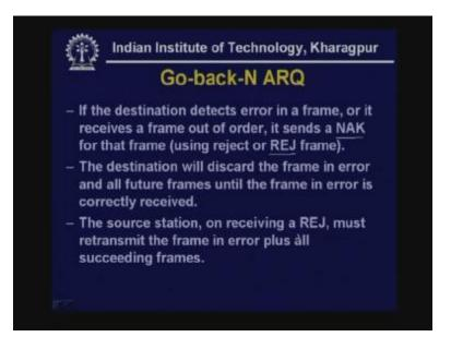
What will happen is the destination will discard the already received frame until a particular frame is received correctly. The source station on receiving REJ reject frame must retransmit the frames in error plus all succeeding frames. Let us see how it actually works. So here it is explain with the help of the diagram.
