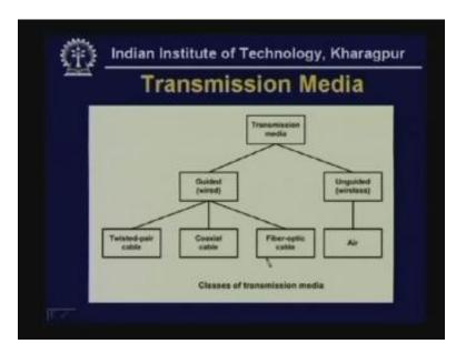
As I said the signal has to be sent through some transmission media. We shall discuss about two different types of transmission media. In fact the transmission media can be broadly divided into two types; one is guided and another is unguided. In case of guided transmission media there are three popular types; twisted pair, coaxial cable and fiber optic cable.
