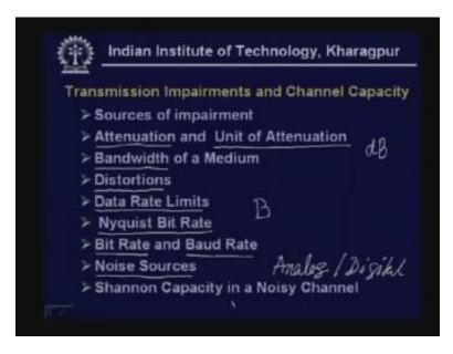
And the rate at which data can be sent will be dependent on the medium and as we shall see there is some data rate limit which can be sent through a medium and which is characterized by Nyquist bit rate. Depending on the bandwidth of the medium the Nyquist bit rate will be decided. We shall we shall discuss in detail about this Nyquist bit rate which is the highest data rate that can be transmitted through the medium.
