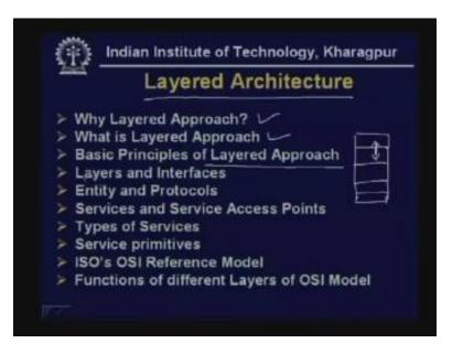
Obviously questions will arise as how these layers interact with each other. So in that context we shall discuss about layers and interfaces and we shall see the various functionalities that is being provided which can be hardware, software or a combination of them which is known as entity and how various protocols, protocols are essentially agreed upon rules and conventions that is being used for communication and how these protocols are used in a layered architecture.
