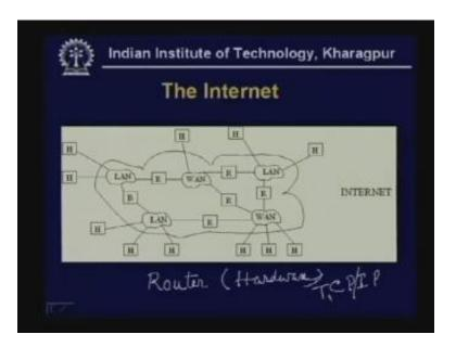
So the single virtual network is widely known as internet which is essentially a network of networks. Question arises as what is the hardware and software that is needed.
