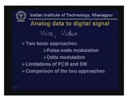
Coming to analog data to digital signals where data is analog in nature such as voice, video etc in such a case you have to convert the analog data into digital form and there are two basic approaches; one is know as PCM Pulse Code Modulation and second one is known as Delta Modulation.
