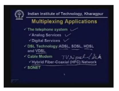
Of course the multiplexing has got very wide applications. and in this lecture series we shall discuss about four important applications and four important applications are telephone system which are used in our day to day life and we shall discuss how using multiplexing technique two different types of services known as analog services and digital services are provided.
