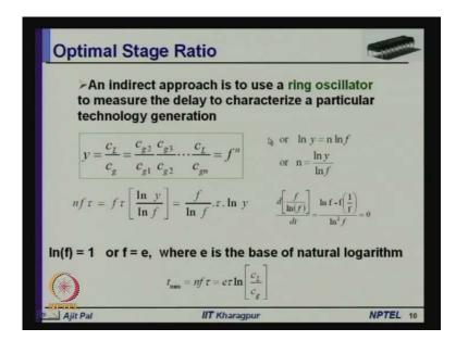
So, you can find out what is the delay this is the delay n f tau you have use n stages with stage ratio of ape ape is the ratio of the C L by I mean that that gate capacitor gate capacitance of the first stage by the minimum gate capacitance. So,n f tau is the value of this then we can differentiate it and make it equal to 0. You know whenever you have to make you have to get the minimum value the standard practice is to differentiate it and equative to 0.
