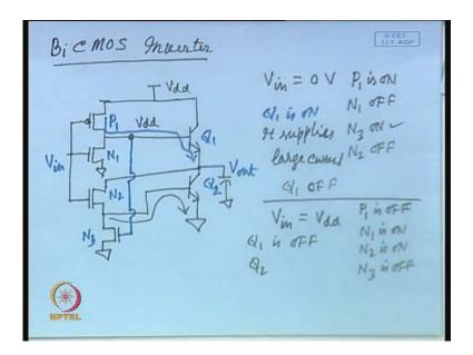
So, this can be modified to realize a bi-C MOS inverter by adding both bipolar and bipolar devices and C MOS devices how it can be done? So, let me draw a BiC MOS inverter actually, you can have different types of realizations of BiC MOS inverter, but I shall I m considering the simplest and the most standard one. So, this is the diagram of that you have got the basic inverter is here.
