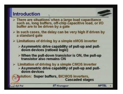
So, we shall discuss all these techniques one after the other. Coming to the introduction, there are situations when a large load capacitance such as long buffers off-size capacitive load or load or IO buffer are to be driven by its gate. See, you are realizing different circuits by using VLSI technique, but you have to drive some off-chip loads.
