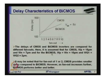
You can see here it has been assumed that for C MOS W p is equal to 15 micron W n is equal to seven micron 2 times and and for the Bi C MOS W p is equal to W n is equal to 10 micron and W Q one is equal to wq 2 is equal to 2 micron so; that means, these are the dimensions of the bi bipolar transistors whereas, these are the dimension of the p MOS and n MOS transistors. So, we have studied the character delay characteristics of a Bi MOS inverter compared to standard C MOS.
