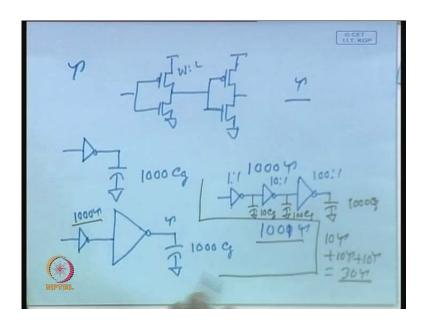
Now let us now consider a situation in which a large capacitive load like output pad is to be driven by a MOS gate and as I have already mentioned typical value can be of the order of hundred picofarads. So, it is quite large. So, if such a load is driven by MOS gate minimum dimension of minimum dimension, then delay can be 10 to the power 3 tau.
