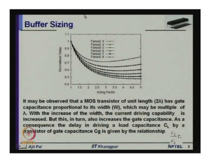
Now let us switch gear and come to the last topic that is your Buffer Sizing you can see here an experiment has been carried out to see the normalized delay for different fan-out and different sizing factor what do you mean by sizing factor? Sizing factor is essentially, how big is the width say for the standard minimum size gate with its 2 lambda.
