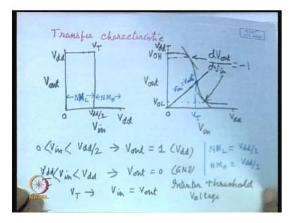
This is the transfer characteristic transfer characteristic. So, the transfer characteristic is essentially represents how exactly the output changes as you change the input. So, this is your input and this is your output. So, how the input gets transferred? I mean input changes the output, that is the represented with help of the transfer characteristic.
