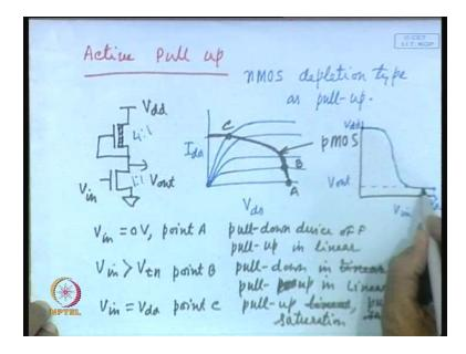
So, active pull-up active pull-up. So, whenever you say active pull-up what do we really mean? We mean that we shall be using some active device. What kind of active device will be using? Obviously, you will you will be using a MOS transistor and we have four alternatives at our disposal. That pull-up device can be a n MOS enhancement type transistor, it can be a n MOS depletion type transistor, it can be a p MOS depletion type transistors. So, you have got four
