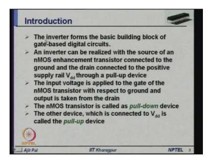
As you know the inverters forms the basic building block of gate-based digital circuits. You you must notice the word gate-based.
