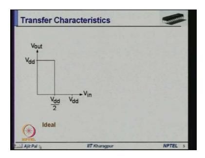
Now, we shall consider the consider a characteristic, important characteristic which is known as transfer characteristic. So, transfer characteristic of a inverter; let me draw it here.
