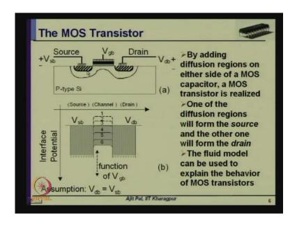
What is the difference between a MOS capacitor and a MOS transistor? As we can see the central portion is essentially the MOS capacitor, and of course on both sides you have got drains and source. So, we can draw it starting from MOS capacitor.
