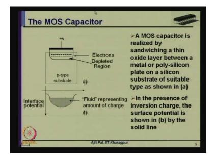
So, based on that fluid model first I shall consider the operation of MOS capacitor, this MOS capacitor is essentially the most elementary building block of MOS transistors or MOS circuits, and a as we have seen a MOS capacitor is realized by sandwiching a thin oxide layer between a metal or poly silicon plate on a silicon substrate of suitable type as show in this figure, let me draw it for your convenience a MOS transistor MOS capacitor.
