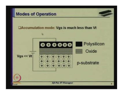
So, after discussing the characteristics of MOS transistors, now we shall focus on another very important aspect, modes of operation. The modes of operation of MOS transistors, we have already explained the operation of a MOS transistor by using fluid model, and we have seen how and when current flow take place, and how the current increases and so on.
