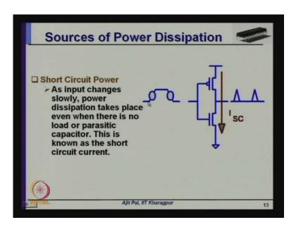
Then comes the short-circuit power, short-circuit power dissipation occurs because of slowly I mean, slow change of the inputs as you can see here input is changing in ACMO circuit as the input changes slowly like this say.
