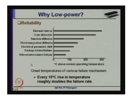
Finally, reliability as I was telling reliability is very important in VLSI chips, and as you can see as the power consumption is increasing temperature will keep on increasing unless you provide proper heat sink to dissipate the power. And you can see there are various failure mechanisms like thermal runaway, gate dielectric, junction diffusion, electro migration diffusion, electrical parameter shift, package related failure, silicones
