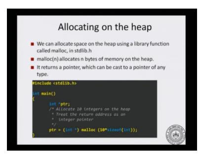
So, how do you allocate things on the heap? There is a standard library function called malloc, in the file std lib dot h which can be used to allocate space on the heap. Roughly, this is what it does, if you ask for malloc n, there n is an positive integer, it will allocate n bytes of memory on the heap and it will return a pointer to the first location of the allocated space. Now, that pointer can be converted to pointer of any type, malloc just allocates n bytes.
