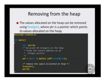
Now, it is nice that you can allocates space on the heap. But, in order to be hygienic, you should also remove the allocated space, once you have done with it. There should be a reverse operation to allocate and that is free, it is in the same library, std lib dot h. And if I just say free ptr and ptr was originally allocated using malloc. Then, it will correctly remove,; however, many bytes were originally allocated.
