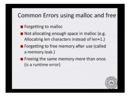
Malloc and free are prone to a lot of errors and a lot of programming errors in c, can be trace back to incorrect use of malloc and free. So, there are some categories of errors for example, you may forget to malloc in the first place. So, you will lead to dangling references or dangling pointers, as we saw in the first example. Now, you could allocate some space. But, you may not allocate enough space, that is a very common error.
