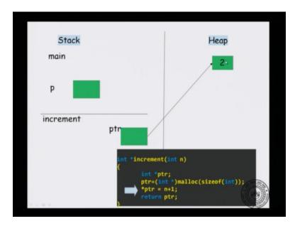
What happens here is that, the increment function ptr points to some location on the heap, using malloc. So, one integer is allocated on the heap and when you say, star ptr equal to n plus 1's, then the location in the heap will contain 2.
