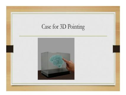
One example of this 3D volumetric display is shown here. So, there is a casing glass casing, within this there is a volumetric display of human brain and you can actually perform gestures to rotate the object to bring some other side to your front as well as you can point to specific locations on the object. So, here in order to point and select you need to make 3D pointing task and we will discuss one model that represents this type of tasks this type of motor behavior to carry out the tasks.
