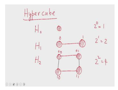
I will define what a hypercube is in this lecture and during the course of the program. We shall see several interconnection networks that are related to hyper cubes, a hypercube of dimension 0 is a single processor without any connection a hypercube of dimension 1 is constructed by taking 2 copies of H 0 and connecting the nodes. And then to construct a hypercube of dimension 2, we take 2 copies of H 1 and connect the corresponding nodes.
