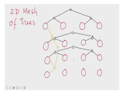
When we have a 2 dimensional mesh of processors instead of connecting them using horizontal and vertical edges, we could connect them using binary trees that hold auxiliary processors for example, you could construct a binary tree over the 1st row of the measure process mesh of processes in this fashion similarly over the 2nd row we construct a binary tree and so on..
