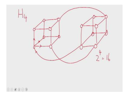
Now, coming on to the 4th dimension we take 2 hyper cubes of dimension 3 and inter connect the corresponding nodes. So, this is this node corresponds to this, these 2 are corresponding nodes they are connected and these 2 are corresponding nodes and they are connected, these 2 are corresponding nodes and they are connected and so on. So, this is how you construct?
