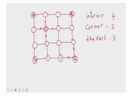
In this case the processes are arranged in a two dimensional array and the processors are interconnected using horizontal edges as well as vertical edges.
