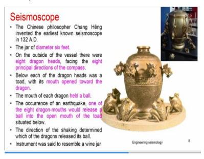
But as on I keep telling you that as on that it is not very successful, okay. So, one of the best or most reliable prediction people have made in the olden days was actually seismoscope, so maybe when we are discussing about the seismometer, we discussed of the seismoscope. So, if you understand how it works basically, it gives warning about soon after earthquake, it gives a warning that which direction earthquake is occurred.
