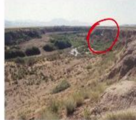
Rotational movement in the banks of Kharrud river resulting from lateral spreading. The white arrow shows the rotation of the earth block.
