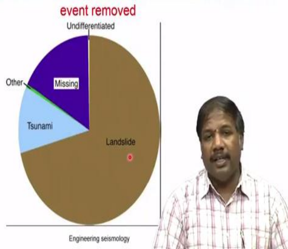
Non-shaking earthquake fatalities for all deadly earthquakes between September 1968 and June 2008, with deaths from the 2004 Sumatra event removed
