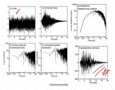
So this is that 6 steps has been broadly explained pictorial way. So this is basically a noise which is simulated based on the duration. Then the; apply here Gaussian window noise filtering so then you will get here this was as it become like this. Then model noise spectrum you can this is the spectrum you will get which is taking into account of your corner frequency all those things then the Fourier amplitude of the same window.
