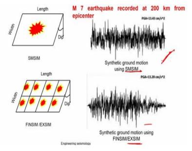
So here the again the entire fault divided as a different segment each has been taken as a single record. So this is the single which is produces one time history. This is the multiple time history clubbed together and finally arrived to this one. So this is basically the SMSIM this is the EXSIM. So this is more suitable for the Peninsular India, this is suitable for the North India above magnitude of 7. You need to have the source information which is required for the input.
