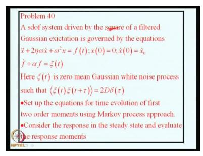
We will begin by considering a problem in random vibration. A single degree of freedom system is driven by a filtered Gaussian excitation and is governed by the equations x double dot 2 eta omega x . + omega square x = f(t) a system starts with some initial conditions and this excitation f(t) is a filtered white noise. That means the white noise x i (t) passes through a first order differential equation filter and this x i (t) 0 mean
