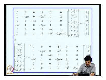
And we can cross this in a metrics form. First, this is the equations for second order moments and we can show that by inverting this. You can get the required values of a steady state response moments mean I have already shown there all 0.
