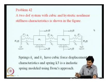
We next consider a fairly complicated problem. This is a problem of a 2 degree freedom system which has both cubic and hysteretic non-linear stiffness characteristics. The springs k 1 and k 2 here have cubic force displacement characteristics. k 3 is an inelastic spring. It has hereditary non-linear characteristics and this is modeled using Bouc's method.
