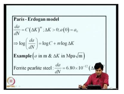
A kind of a dimensional analysis can be performed and the structure of this law can be identified in it is identified in this form a several non dimensional parameters here and one of the model that is popularly used is known as the Paris Erdogan model where we assume that the equation is d a by d N is C delta K to the power of m delta K greater than 0 a of 0 is a naught that is a initial crack length.
