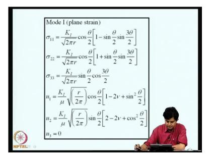
So, if stress exists yield stress, the linear behavior seizes. Similarly, if SIF exceeds critical SIF, the cracks propagates. In terms of stress intensity factor, the stress fields and displacement fields in r theta coordinate can be summarized as shown here.
