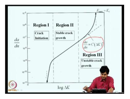
Now, experimentally, it is observed that the rate at which crack propagates, suppose a is a crack length and n is a number of cyclic cycles of loading, d a by d n if you plot as a function of log delta K, delta K is K is the stress intensity factor delta K is a increment.
