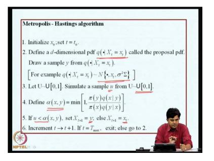
There is an algorithm by the name Metropolis-Hastings algorithm, which helps us to form the Markov chain, which has the target stationary probability distribution function. So, the algorithm itself is quiet simple; so what we do is, we initialize x naught and set t to t naught. Then we define a d-dimensional probability density function denoted by q and this is known as proposal probability density function, and we draw a sample from this proposal density function.
