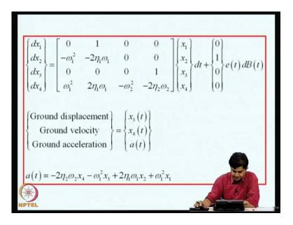
So, by using a vector x 1, x 2, x 3, x 4 as y 1, y 1 dot, y 2, y 2 dot, we can get the equation in the stretch phase form and this can be further simplified, further recast into the SDE - stochastic differential equation – form, in terms of increments of Brownian motion process. There is only 1 white noise driving component here, therefore the b vector is simply 0 1 0 0 and this, a, is the matrix, this matrix into x 1, x 2, x 3, x 4.
