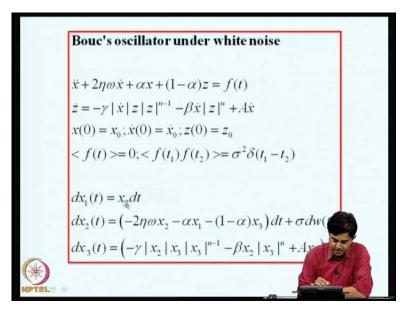
One more example to the set of examples that I considered, we will consider a system in which non-linearity is hereditary and one of the models for that is in terms of, what is known as, Bouc's oscillators. Then here, the non-linearity arises through an internal variable z, which is governed by an additional first order differential equation.
