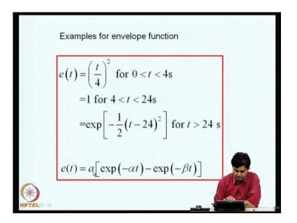
Now, we will pass this acceleration through the high pass filter to remove singularity at the 0th frequency and this is the filter equation for that in the time domain. Now, the envelope that I was mentioning e of t, there are various models proposed, one of the models is as shown here. There is a rise time upto about 4 seconds and the envelope rises, as rises quadratically, and it remains constant for about 20 second, which is a strong motion phase and then there is an exponential decay.
