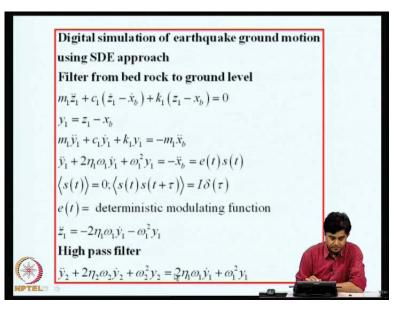
So, this is where we can consider the application of the stochastic differential equation approach to simulate samples of ground accelerations.
