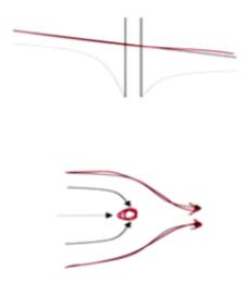
So, obviously you know we are going to have a gradient here and that is what we see out here, right, so in that case if I pump it in from the same location, at the same flow rate, you see that you know there are flow lines; groundwater flow lines which are not going to be captured by the pump here, right. So, the key aspect obviously that we need to consider is where do I place the pump and so on and so forth.
